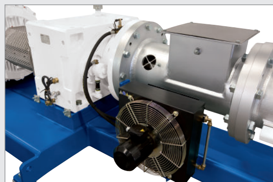
Drive with combined gearbox-bearing assembly
